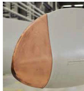
Top: Copper strip installed on blade
