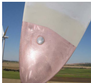
Copper cap before surface finishing
