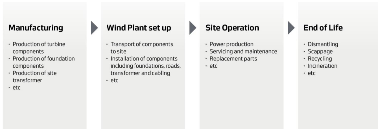
Figure 4: Life cycle stages of a typical onshore wind plant including typical activities
