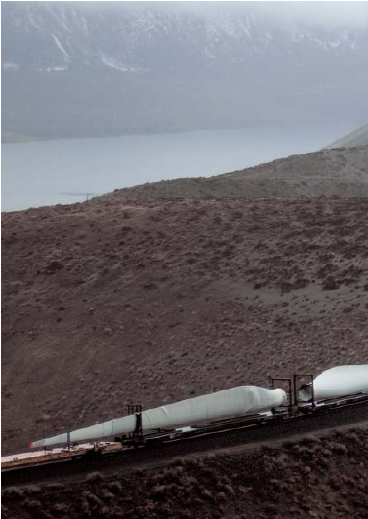
In 2003, Vestas transported both blades and nacelles by train to a range of sites in the United States.
